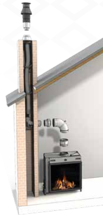
Via the roof • flexible pipe in the chimney
