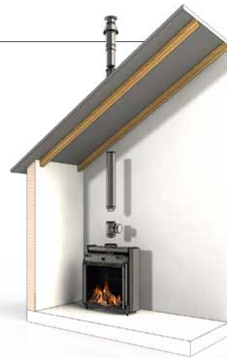
Via roof (pitched) • straight or with bends
