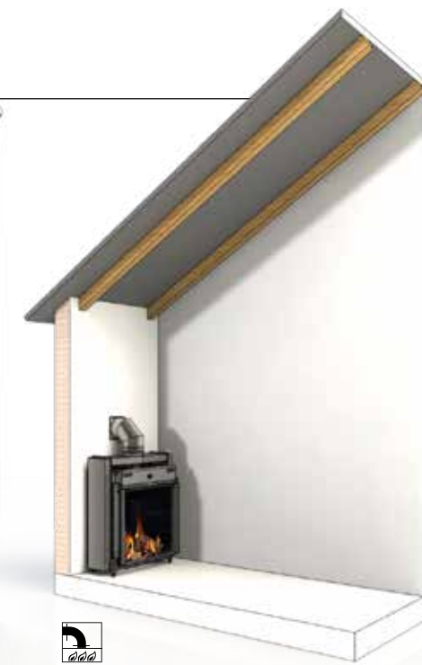
Via wall • directly on the fire with a 90° bend to the outside • possibly on a large part of the range
